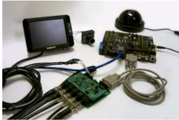
Figure 1: IP network video server allows the digitization of up to 4 channels of analog NTSC video from off-the-shelf CCTV cameras and serving out the data onto an 10/100BaseT Ethernet network.
