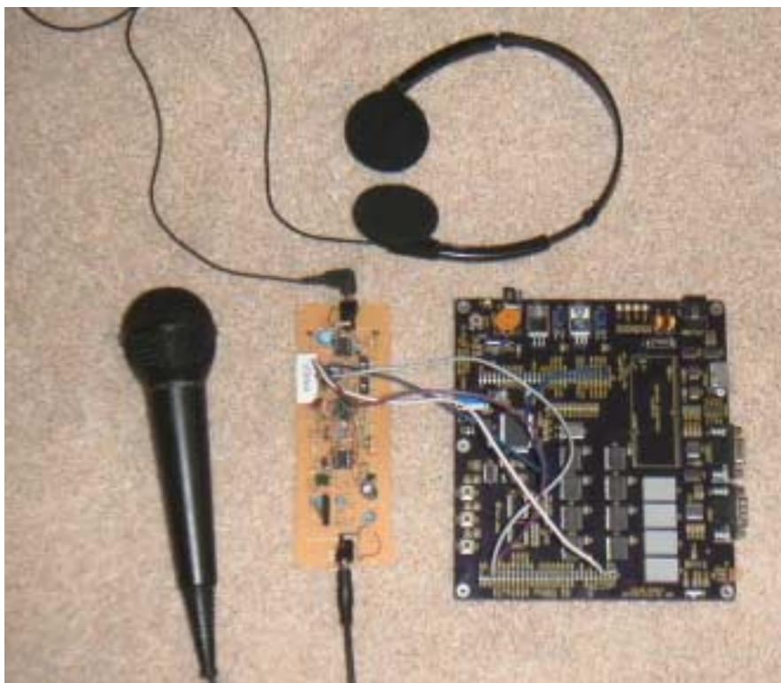
Photo 2 – Entire system consisting of Z8 Encore Development Board, Analog Board, microphone, and headphone.
