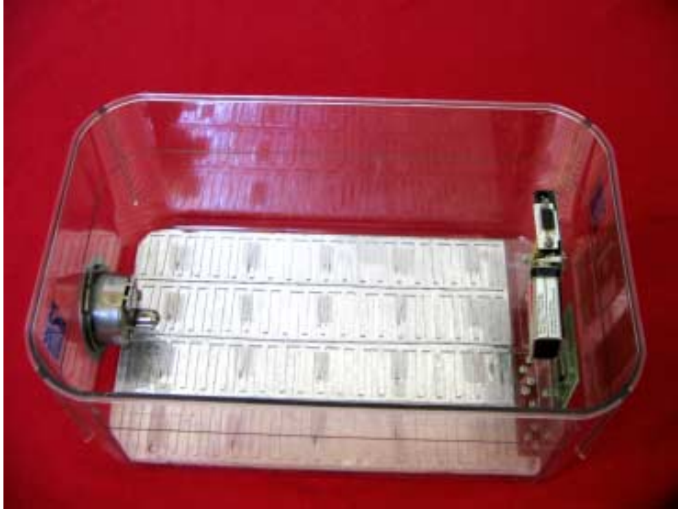
The data acquisition unit placed on the bottom of the mice cage.
