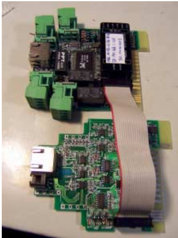
Figure9 Connecting main board and expansion board
